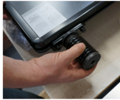
2. Screw springs onto base of frame.
